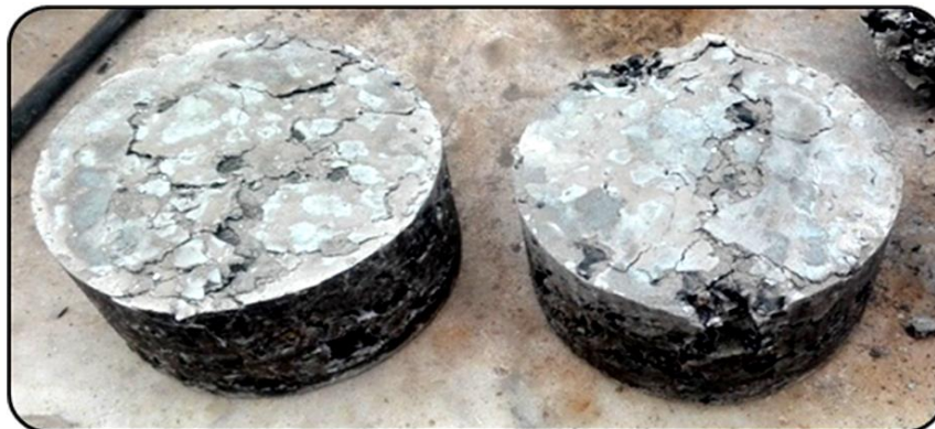
Fig. 14: Failure shapes after Marshall test
