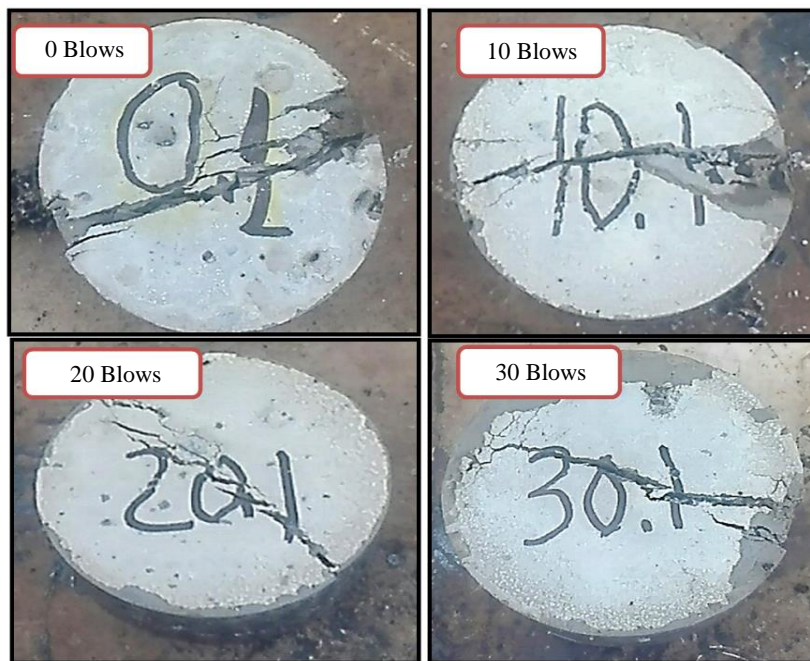
Fig. 16: Failure shapes after indirect tensile strength test
