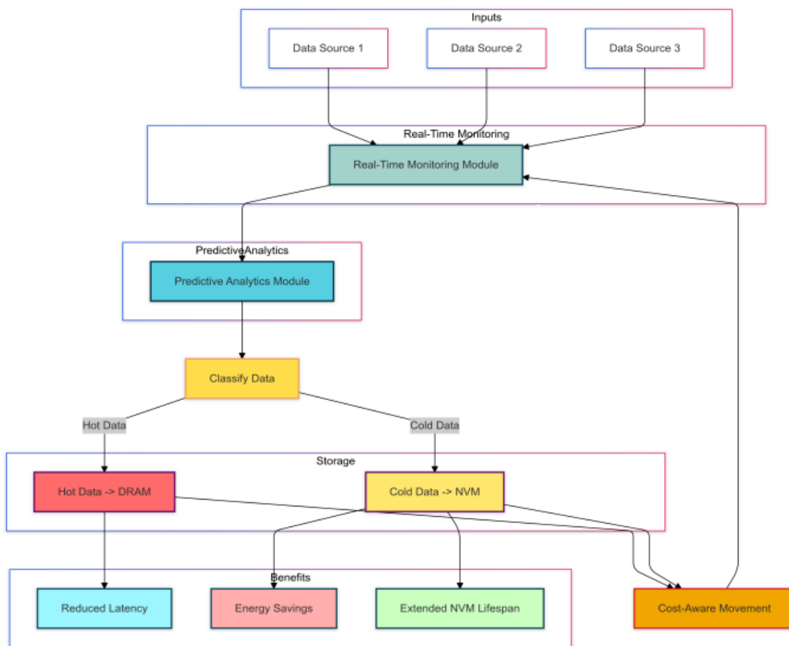
Fig. 1: Proposed Hybrid Memory Architecture for Adaptive Data Placement and Energy Optimization
