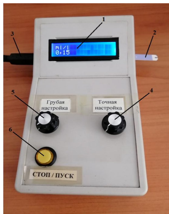
Fig. 1: Biosensor assembly: 1 - display; 2 - sensor; 3 - external power cord; 4 - biosensor fine tuning; 5 - biosensor coarse tuning; biosensor power button
