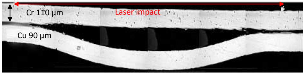
Fig. 3: Cross section analysis of a Cr 110 μm-Cu 90 μm sample after LASAT test
